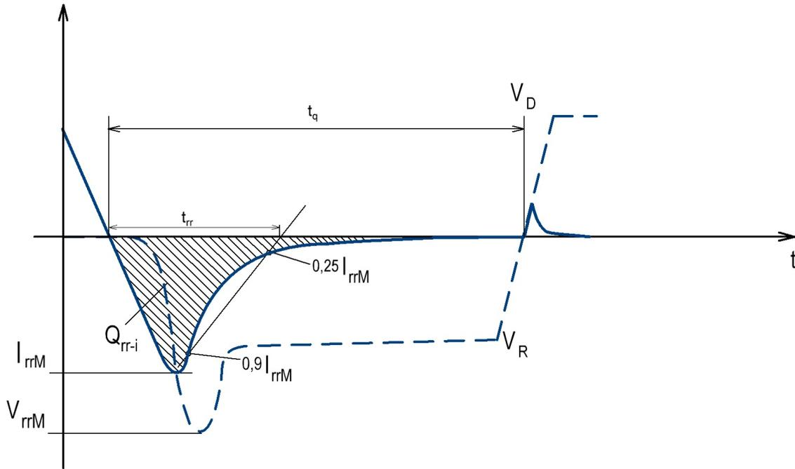
Figure 16. Reverse recovery and turn-off process of a thyristor.
