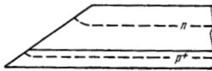
Figure 3. Edge bevel of a diode semiconductor element.
