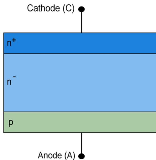
Figure 2. Typical cross-section of the semiconductor structure of a power diode with p-n junction.
