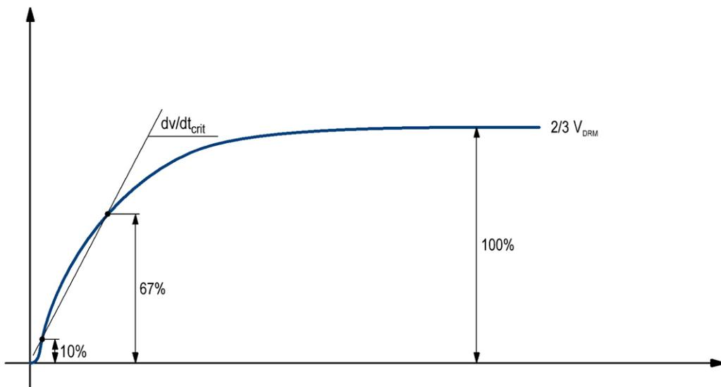
Figure 15. Determining  $dv/dt$
