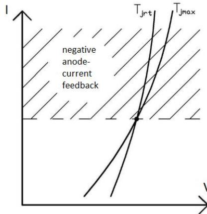
Figure 32. Point of temperature inversion and negative feedback zone.
