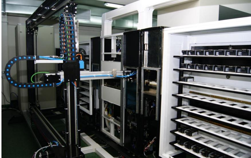
Figure 28. Automated complex for measurements of power semiconductor modules
