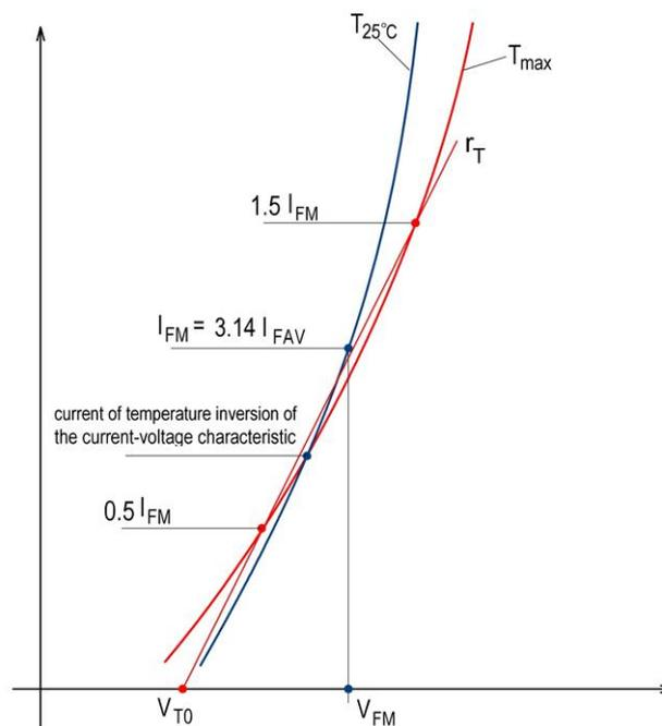
Figure 6. Typical forward current-voltage curve of a power diode.
