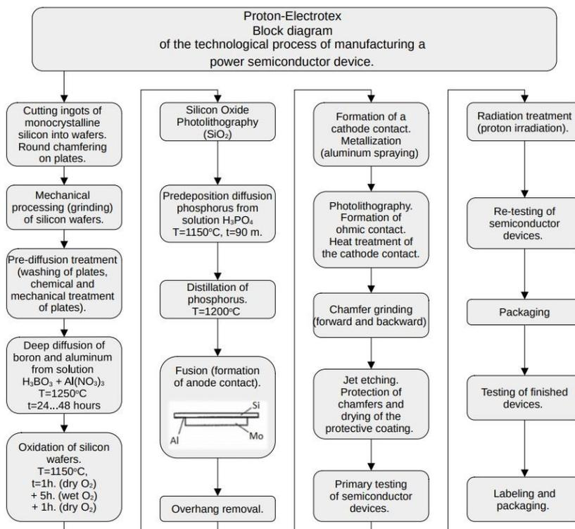
Figure 26. Block diagram of the manufacturing process for a power semiconductor thyristor.
