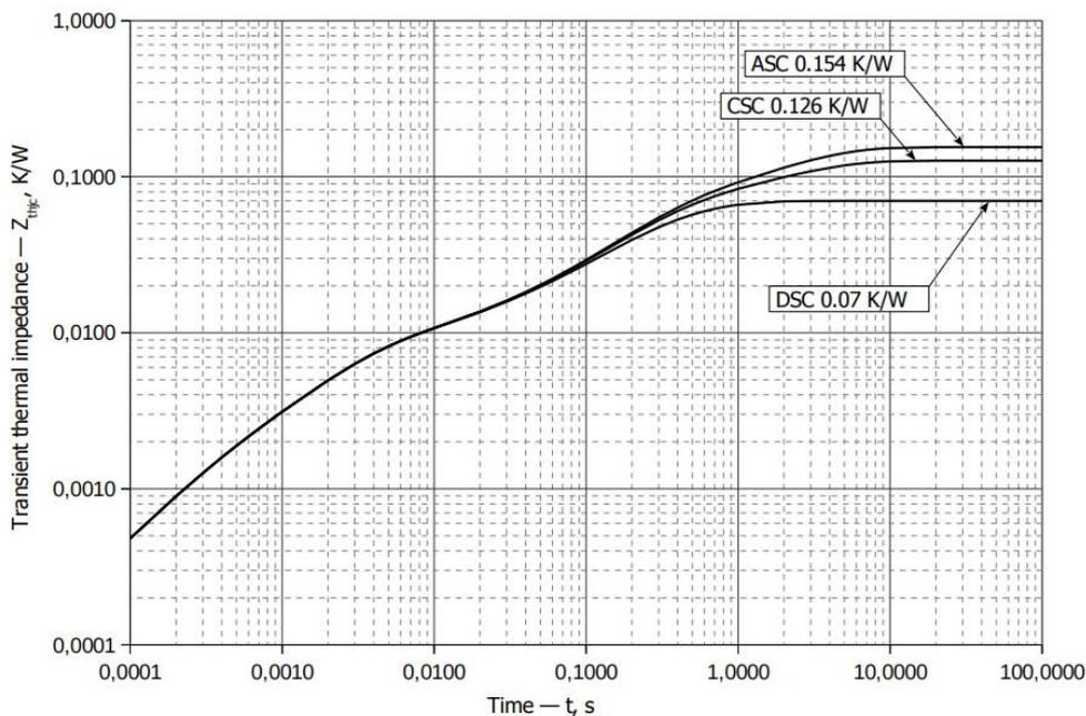
Figure 23. Time dependence of transient thermal resistance.
