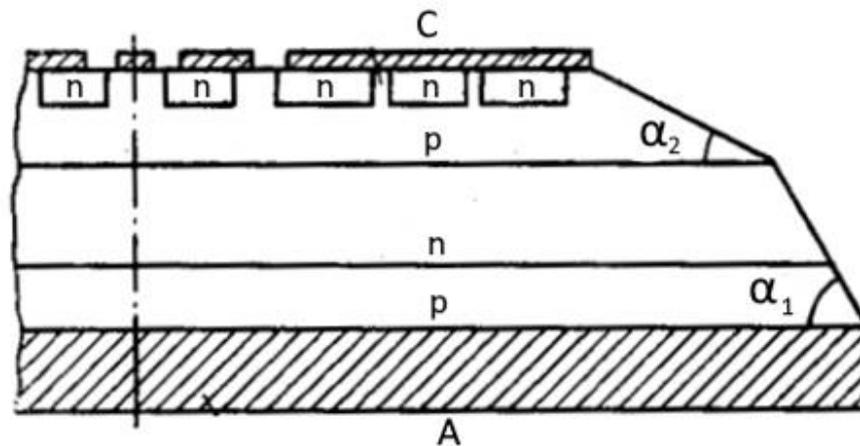
Figure 13. Typical profile of a power thyristor's semiconductor element.
