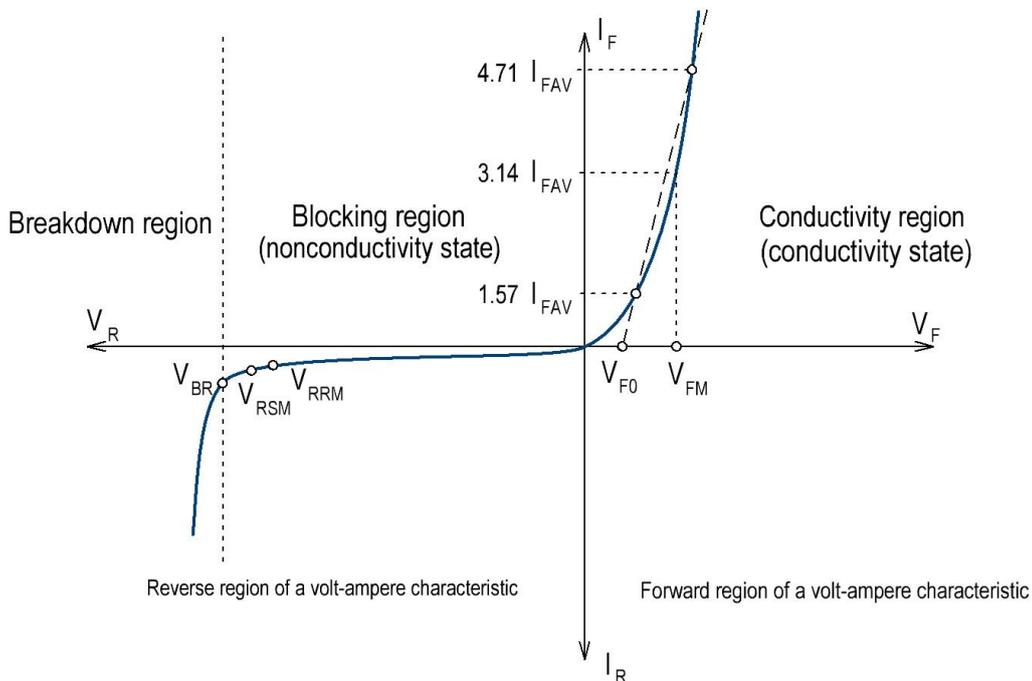
Figure 4. Typical current-voltage curve of a diode.
