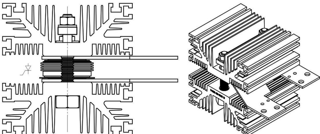
Figure 33. An assembly example for a disc thyristor and a heatsink.
