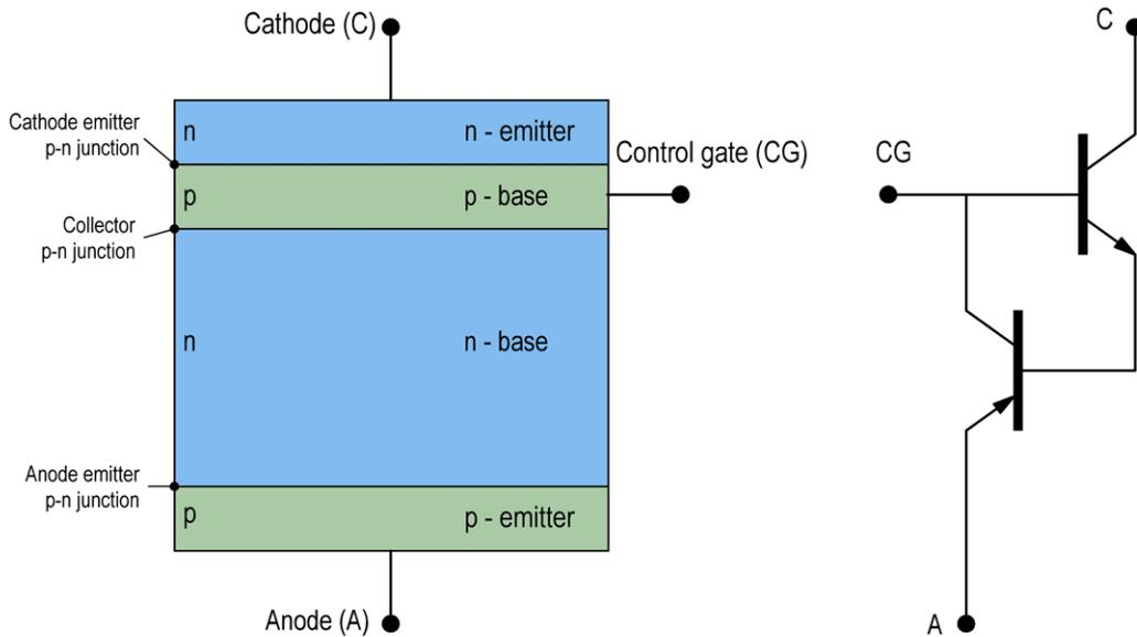
Figure 9. Cross-section of a thyristor's semiconductor structure and its circuit diagram.
