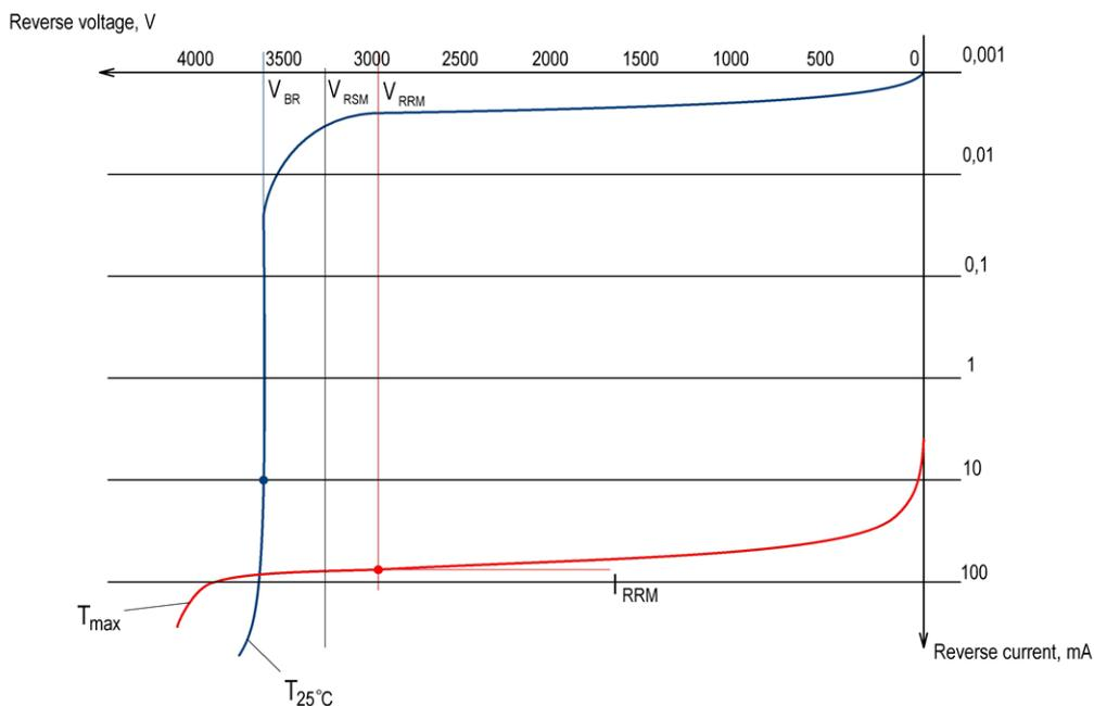
Figure 5. Typical current-voltage curve in logarithm scale.
