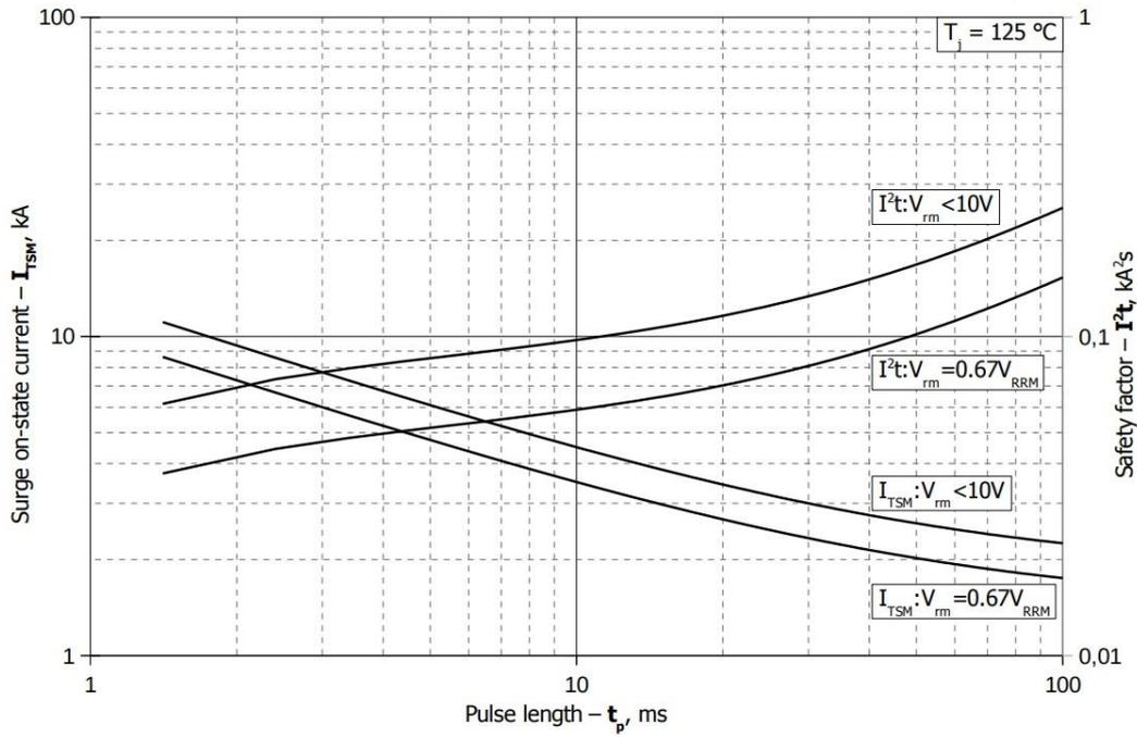
Figure 24. Relation between the maximal amplitude of surge current in open state  $I_{TSM}$ , protective factor  $I^2t$  and impulse duration  $t_p$ .
