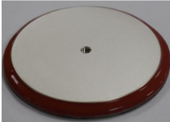
Figure 22. Housingless welding diodes.
