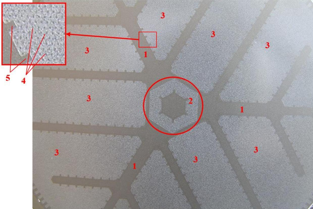
Figure 12. Topology of a semiconductor structure of a modern thyristor (with removed cathode metallization): 1 - branched p-gate region, 2 - auxiliary thyristor, 3 - cathode region of the main thyristor, 4 - p-region of distributed shunt elements, 5 - p-region of edge shunt elements of a branched gate electrode.
