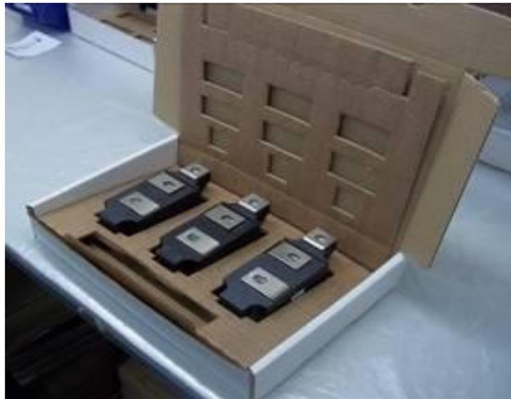
Figure 36. Modules in internal packaging
