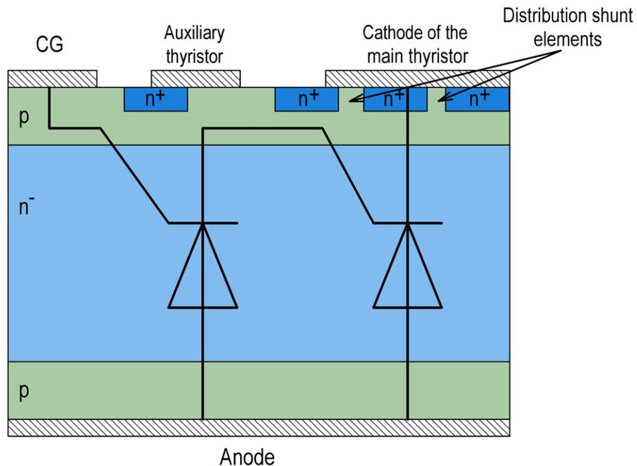
Figure 11. Cross-section of a thyristor's semiconductor structure.
