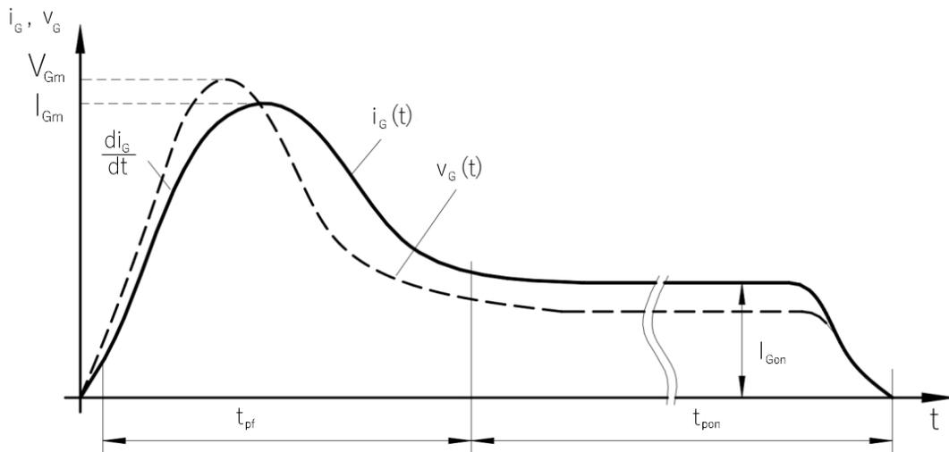
Figure 31. Diagram of current and voltage in gate circuit.
