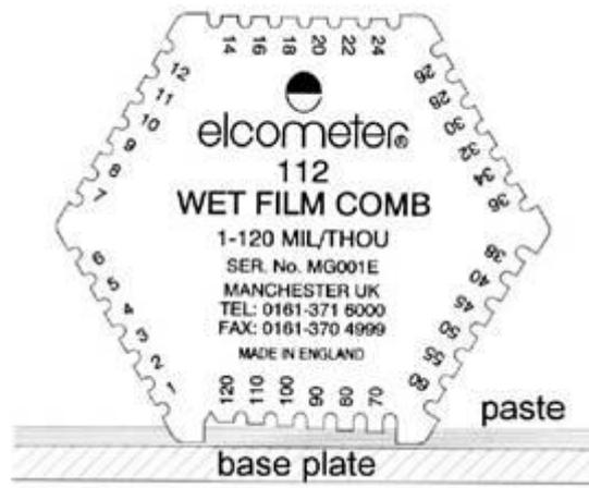
Figure 34. Wet film comb used to measure the thickness of thermal paste.
