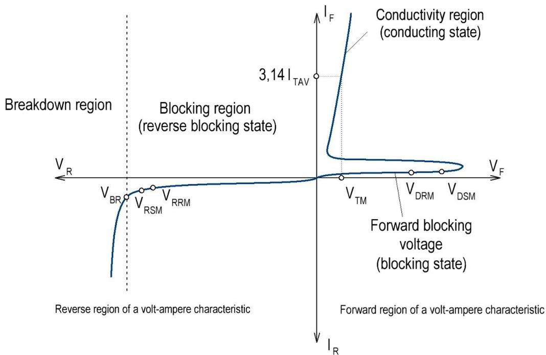
Figure 14. Voltage-current curve of a thyristor.
