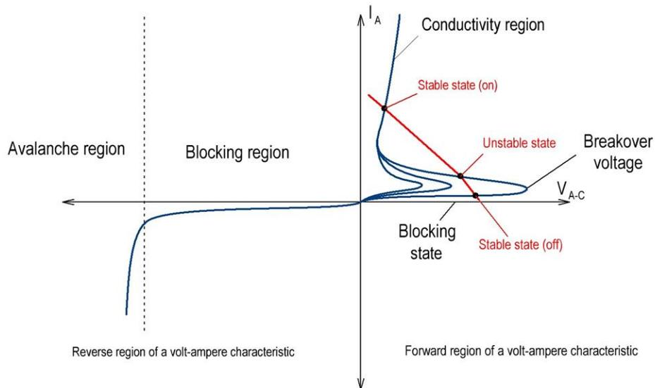
Figure 10. Typical current-voltage curve of a thyristor.
