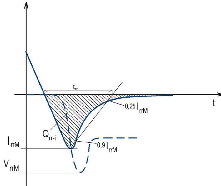
Figure 7. Reverse recovery of a diode with p-n junction.
