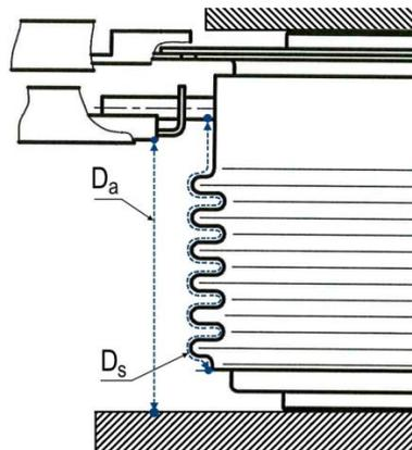
Figure 25. Total and straightened distances between the anode and the gate electrode of a disc thyristor.
